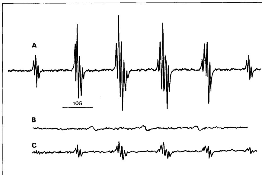
FIGURE 1 The ESR spectrum obtained from 500 \mu\text{M} procarbazine (A) in the presence of DBNSB spin trap (2 mg/ml) with HL60 cells ( 5 \times 10^6 cells/ml) in PBS; (B) same as (A) except no drug was present; and (C) same as (A) except no cell was present. The ESR settings were: field = 3480 G; microwave power = 20. mW; scan range = 100 G; scan time = 500 sec; modulation amplitude = 1.0 G; time constant = 1.25 sec, and the receiver gain was 2.5 \times 10^5 . The ESR parameters for the DBNSB-CH 3 adduct are a^N = 14.5 G; a^H = 13.7 G; a_m^H = 0.7 G.
